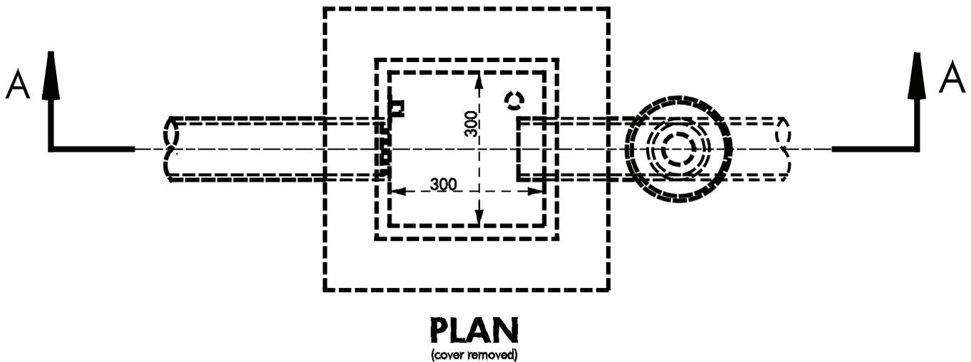
1. 32mm x 32mm x 25mm deep polyvinyl chloride (P.V.C) bracket to be fitted as close as practical to the outlet.
