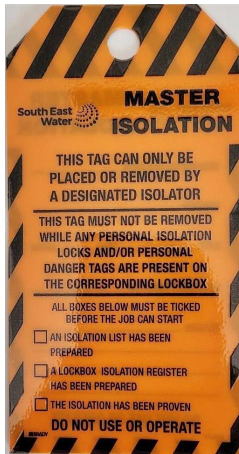
Figure 4: Example Master Isolation Tag
