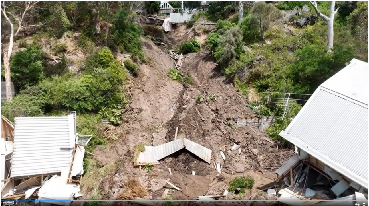
Figure 11: Drone footage taken from toe of failure, illustrating the 'bowl' shaped failure within the upper slope.
