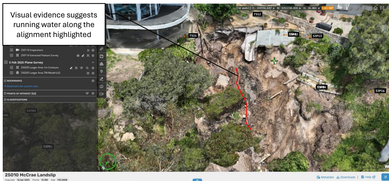
Figure 15: Detail of the presumed slip area with the red line an annotation of possible running water at the time of drone footage.
