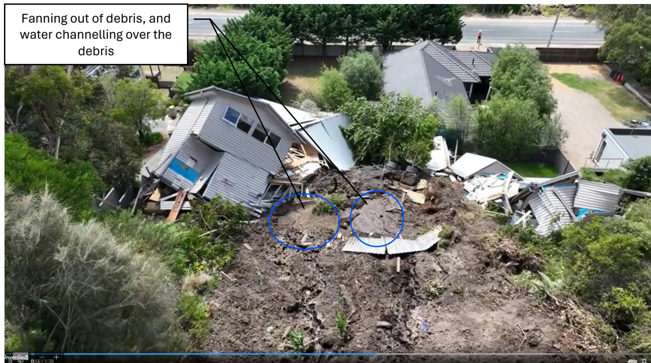
Figure 18: Drone footage, showing the toe debris.
