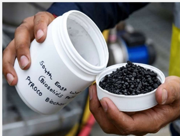
Figure 11. Figure holding container of biosolids, by-product of the pyrolysis (PYROCO) process
